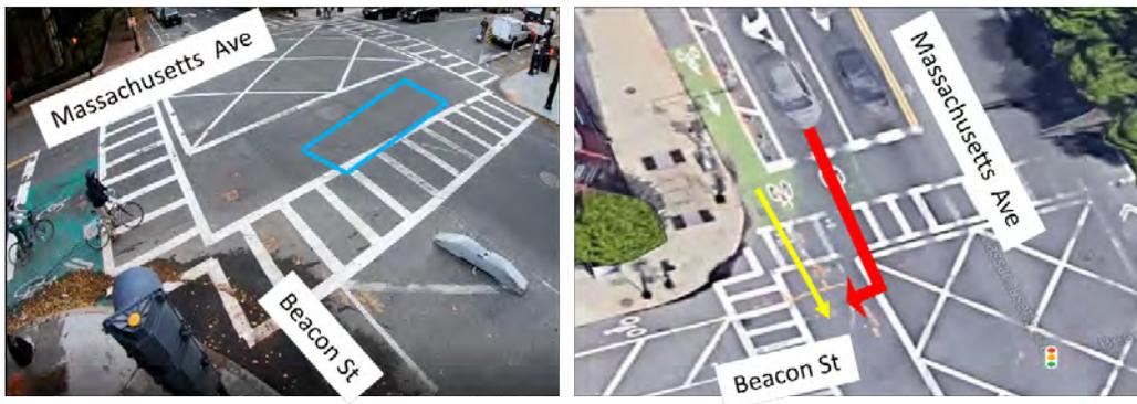
Figure 9: Massachusetts Avenue at Beacon Street (Boston, MA). [Segment: protected bike lane; Intersection: bike box and crossing markings]
