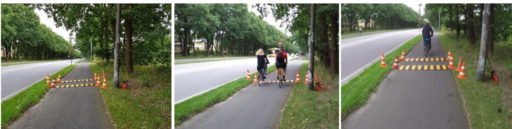
50 Figure 2. Narrowing of cycle track and lateral displacement of cyclist using delineators. Two different settings were 51 tested. On the left (2.1), the bicycle area is narrowed from the left with 2 delineators and then from the right with 3 52 delineators with a gap between delineators of 4 m. On the right (2.2) the bicycle area is narrowed with 3 pairs of 53 delineators spaced 4 m apart, first from the left then from the right and then again from left.
