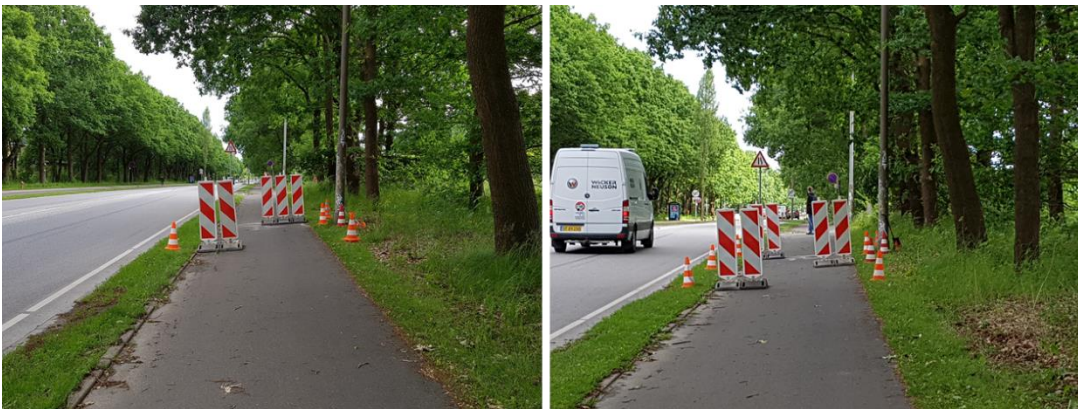
50 Figure 2. Narrowing of cycle track and lateral displacement of cyclist using delineators. Two different settings were 51 tested. On the left (2.1), the bicycle area is narrowed from the left with 2 delineators and then from the right with 3 52 delineators with a gap between delineators of 4 m. On the right (2.2) the bicycle area is narrowed with 3 pairs of 53 delineators spaced 4 m apart, first from the left then from the right and then again from left.
