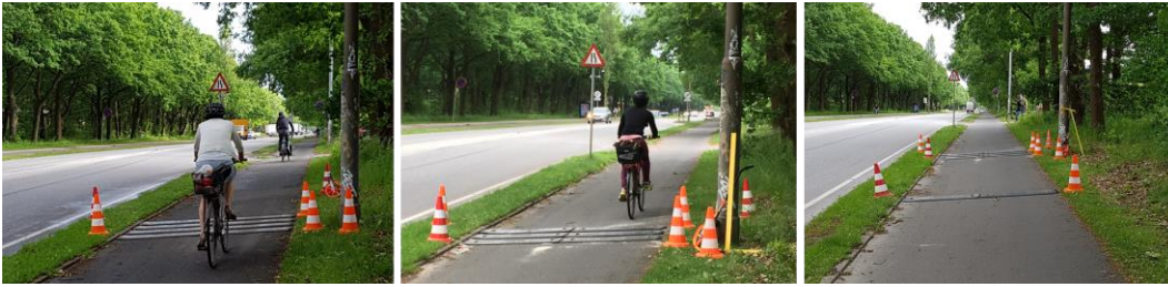
45 Figure 1. Black portable rumble strips. Three different settings were tested. The left design (1.1) has 4 strips spaced 20 46 cm apart. The design in the middle (1.2) has 3 strips spaced 20 cm apart. The design on the right (1.3) has 4 strips 47 where the distance between the first two is 6 m, while the distance between the last three is 20 cm.
